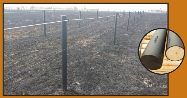
The Woodshield posts went through the same intensity of fire as the treated timber posts. The Woodshield posts have no splinters or cracks for the flame to catch on and there are no chemicals to fuel the fire.
