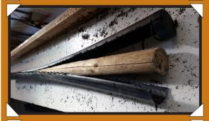
Peel the polymer off the untreated timber post like peeling a banana
