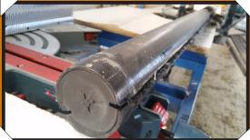
Take a circular saw and make a cut down the length of the post on each side
