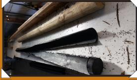
The chemically free timber is seperated from the polymer outer
